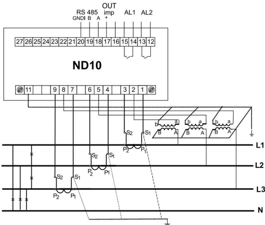
Caution: It is recommended to connect ND10 meters (RS-485) to a computer with a shielded wire. A shield should be connected to ground in a single point. Shielded wire must be used in case there are many interferences in the environment.
