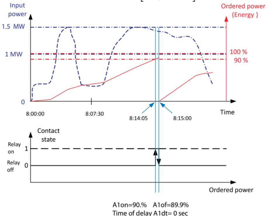
Fig. 9 shows an example of how the consumed ordered active power parameter can be used to alarm activation. Delay time is set at 0 seconds (**A1dt**).
