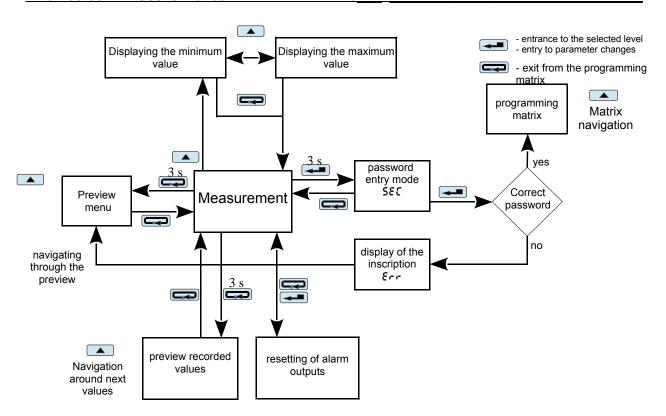
Fig. 7 The NA5Plus meter operation algorithm
