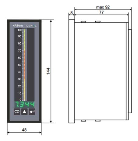
Fig. 2: Dimensions of the meter
