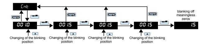
Example of changing the value of the selected parameter with a fixed decimal point (numeric parameter)
