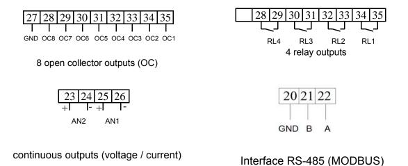
Fig. 5: Output signals connection method
