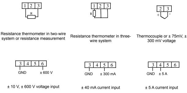
Fig. 4: Input signals connection method
