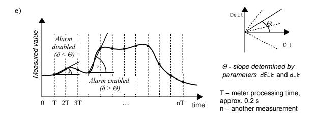
Fig. 10 Alarm types a, b - normal; c - switched off; d - switched on; e - delt
