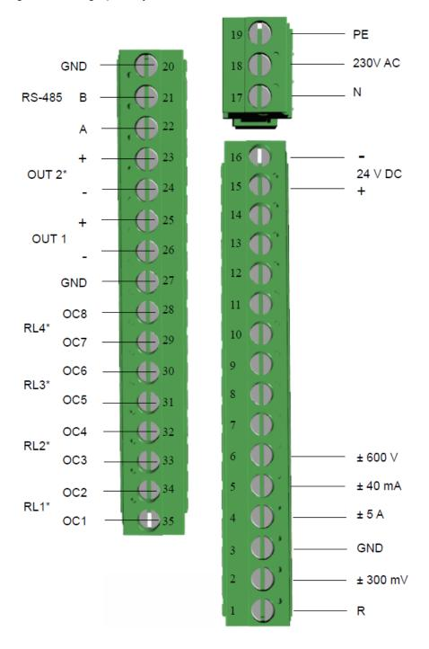
Fig. 3: Electrical connections of NA5Plus meter
